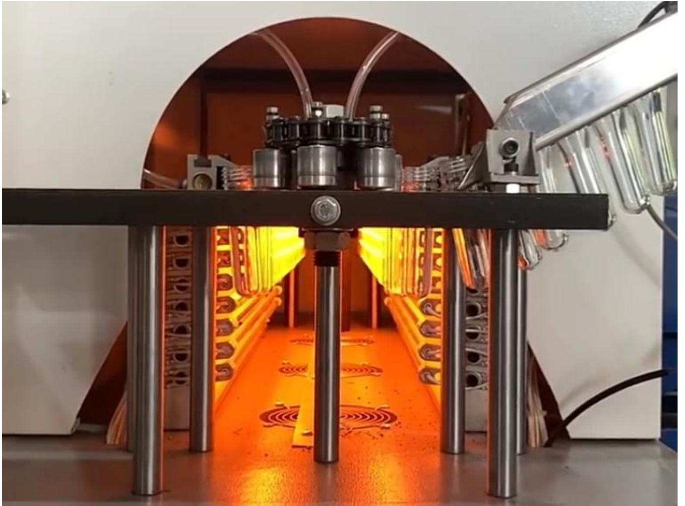
UV Resin and IR Heating curing
