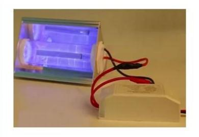
222 nm lamp both side connected with a ballast input. And out contact with a suitable adapter to suit for city Electricity.
